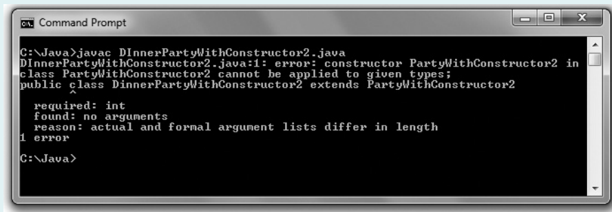
Figure 10-11 Error message generated when compiling the DinnerPartyWithConstructor2 class
