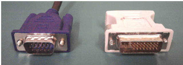
FIGURE 5.4 VGA connectors (left) were common in years past and are still available today; DVI connectors (right) are common on newer monitors and video cards.
