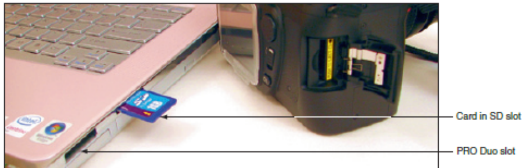
Figure 7-14 This laptop has two flash memory card slots
