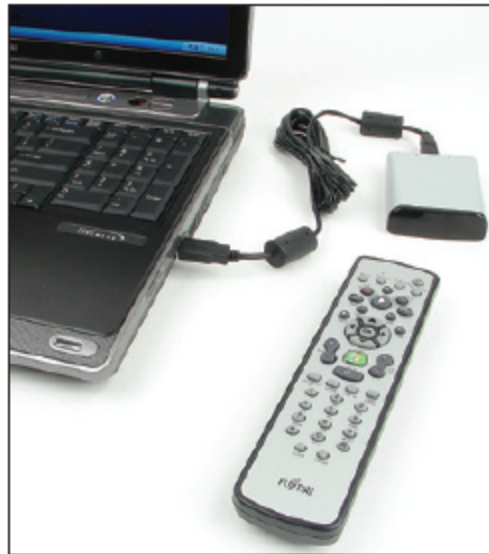
Figure 7-4 This remote control is an infrared device that uses an IR transceiver connected to a laptop by way of USB port
