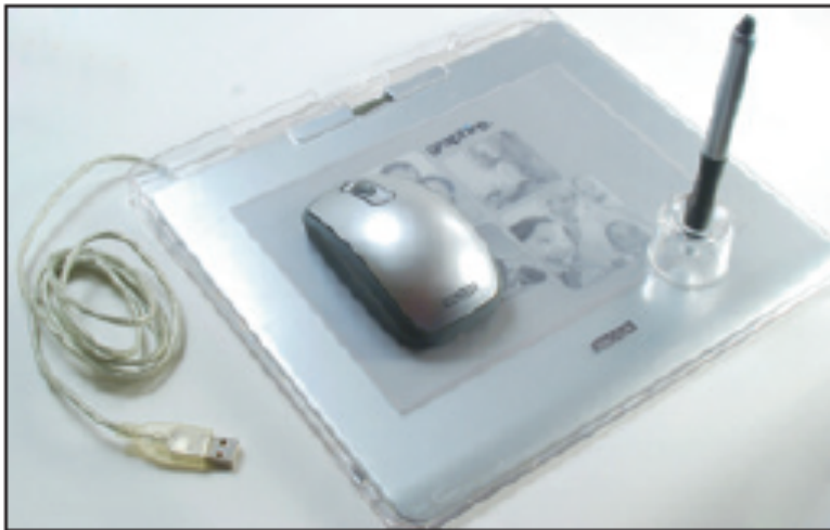
Figure 7-19 A graphics tablet and Stylus are used to digitize a hand drawing
