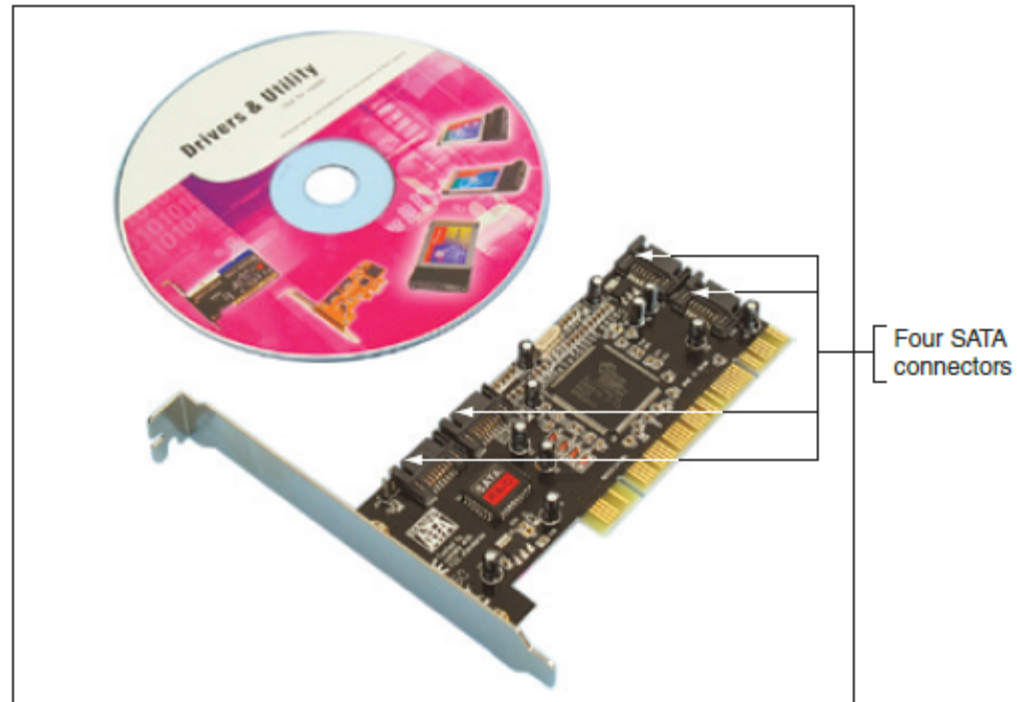
Figure 6-28 RAID controller card provides four SATA internal connectors
