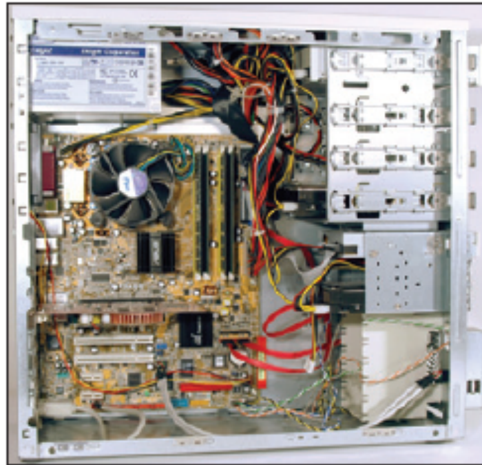
Figure 5-23 Use cable ties to hold cables out of the way of fans and airflow
