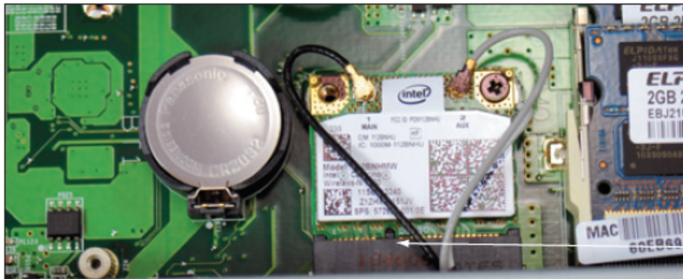
Figure 3-23 Mini PCIe slot with a wireless Mini PCIe card installed
