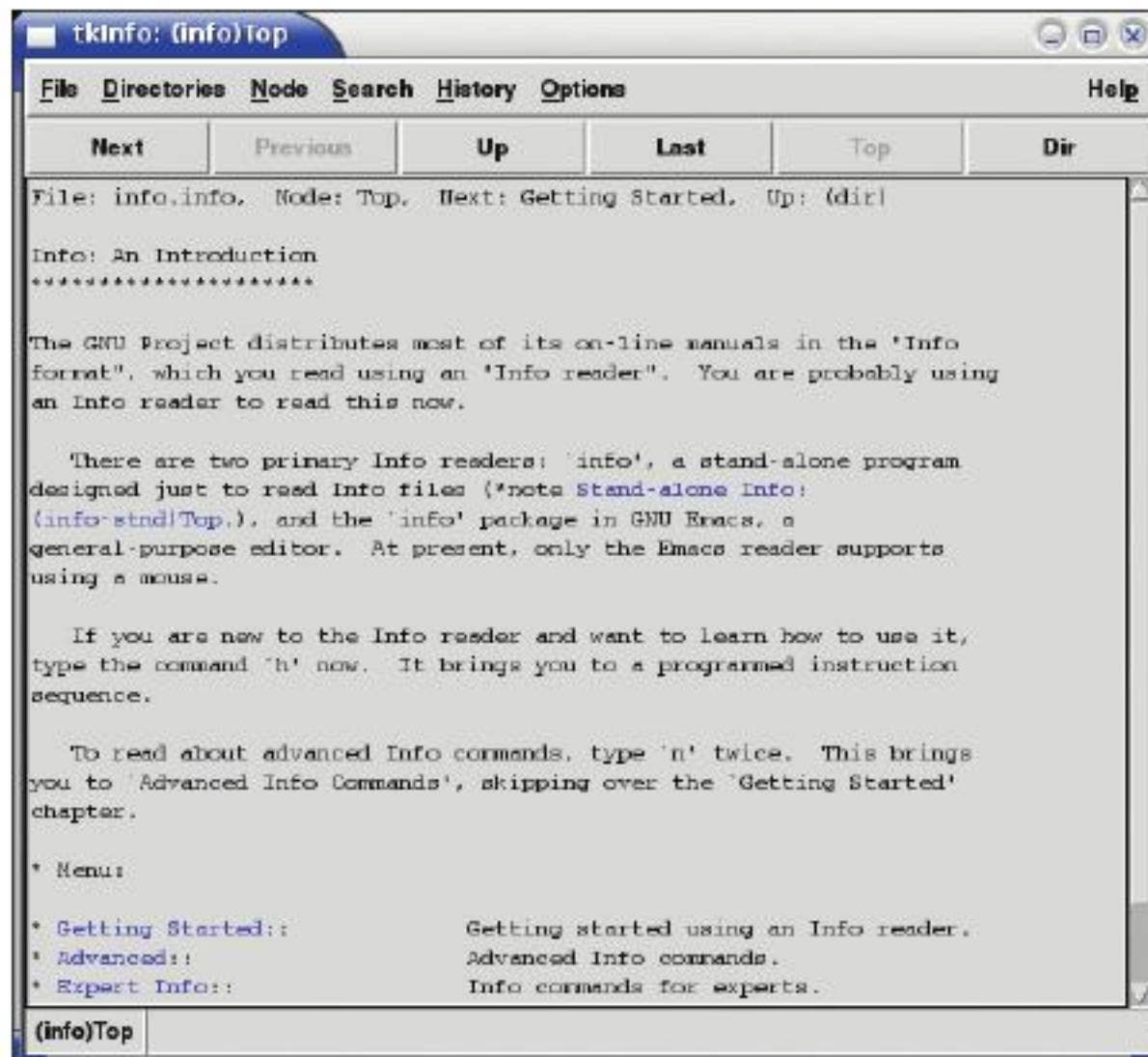
FIGURE 8.2 GUI info page browsers can make this form of documentation accessible to those who are uncomfortable with the command line.
