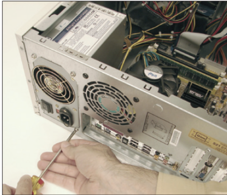
Figure 2-16 Removing the power supply mounting screws
