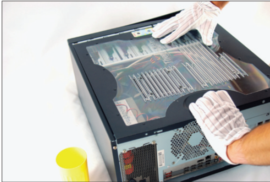
Figure 2-5 Slide the panel to the rear of the case
