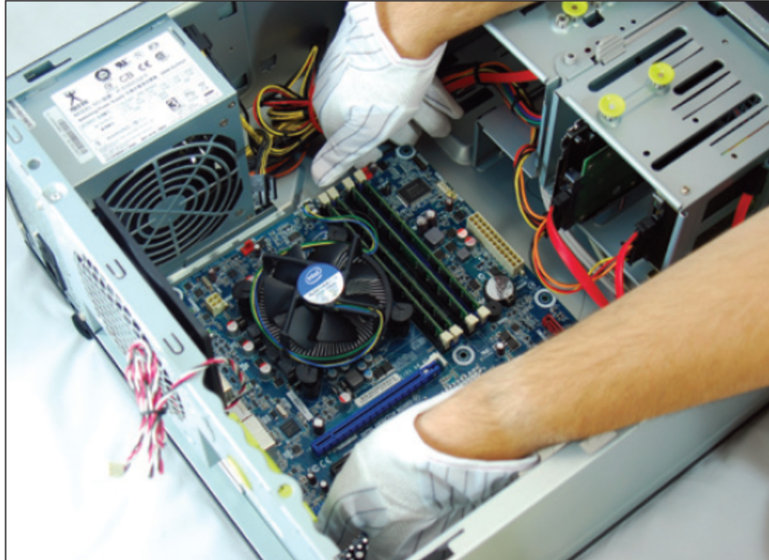
Figure 2-15 Remove the motherboard from the case
