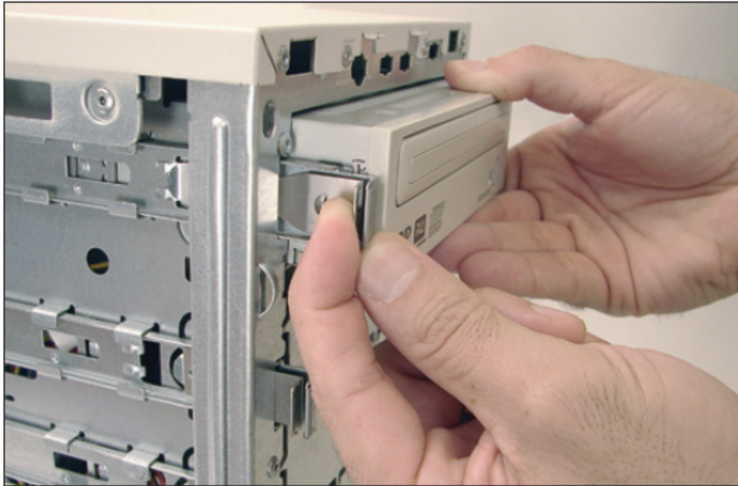
Figure 2-17 To remove this CD drive, first pull the clip forward to release the drive from the bay
