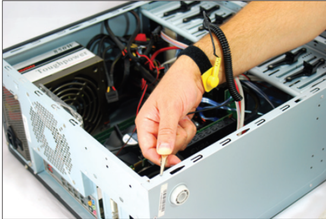
Figure 2-8 Attach the alligator clip of your ground bracelet to the side of the computer case
