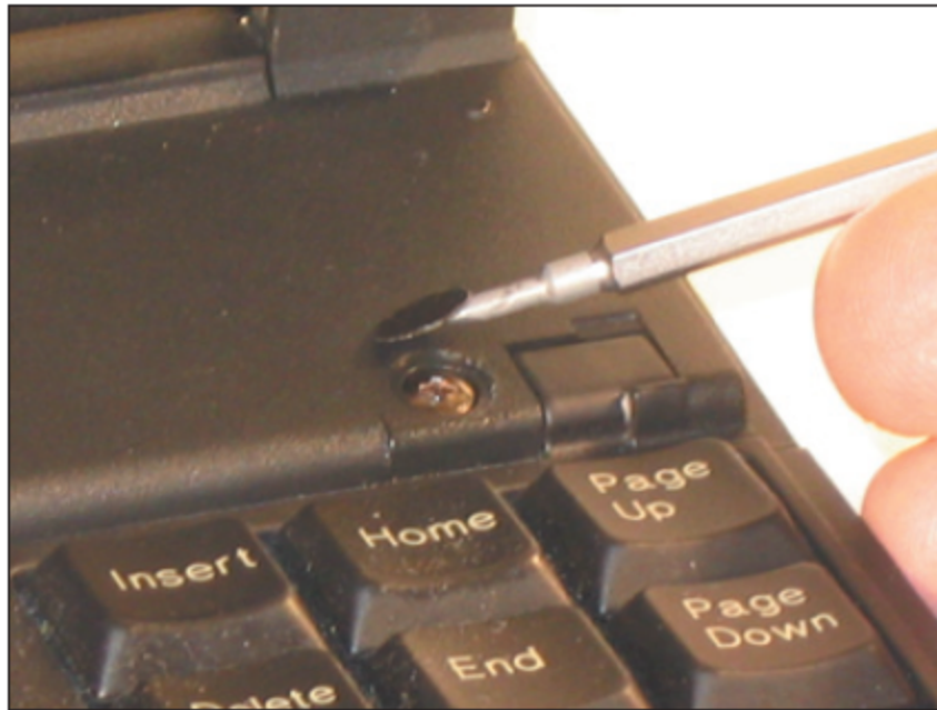
Figure 2-38 Use a small screwdriver or dental pick to pry up the plastic cover hiding a screw
