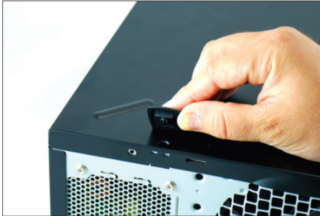
Figure 2-4 On this system, clips hold the side panel in place
