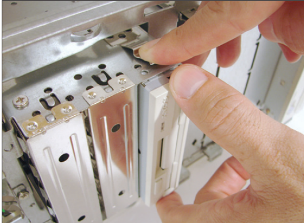
Figure 2-18 Push down on the clip and then slide the removable bay forward and out of the case
