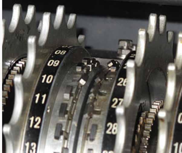
Cams on wheels 9 and 10 showing their raised (active) and lowered (inactive) positions.
